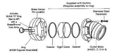
When shipped, the sight glass, gaskets, bolts and washers are attached to the outlet in a plastic bag and must be installed to the mating #4500/4500V ring. The ring is supplied assembled. To install the sight glass and attach the drop adapter, proceed as follows:
