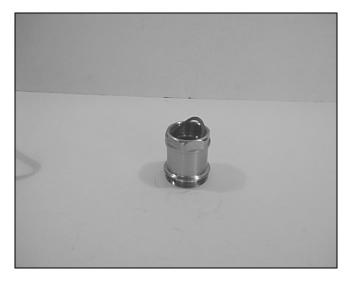
Place a new flat seal (pos.29) on the swivel sleeve. (Not needed when NPT-thread)
