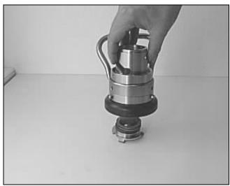
Place the coupling body over the driving plate packet. Grab the piston guide and turn the unit upside down.
