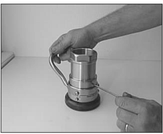
Use Loctite® 243and screw the lock screw into the swivel ring without any force! Risk to deform the ball bearing!
