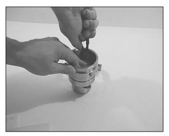
Press down and turn the driving plate to the position where the driving plate heels are placed under the rollers.
