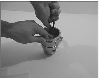
Turn the driving plate to the position where the recess ends up under the rollers.
