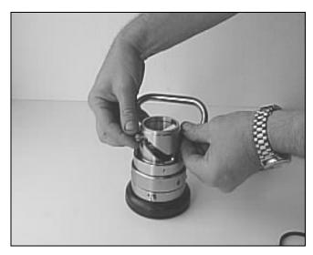
Assemble the two shafts for piston guide.
