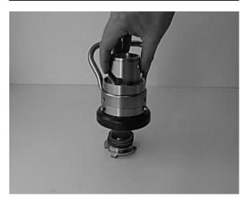
Turn back the unit and remove the driving plate packet from the coupling body.
