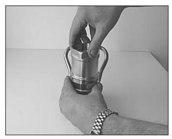
Place the swivel sleeve over the coupling body and screw in the swivel sleeve.
