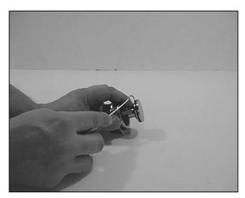
Change the O-ring (pos.3) on the piston. Use grease on the new O-ring. Make sure that the O-ring doesn't get twisted when mounting.
