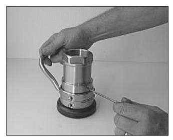
Begin with unscrewing and remove the lock screw from the swivel ring.
