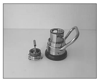
Before the coupling body places on the driving plate packet, make sure that the part where the upper cam curve ends, shall be placed exactly over one roll, and the heel on the driving plate packet should be placed under the hole for the shaft.
