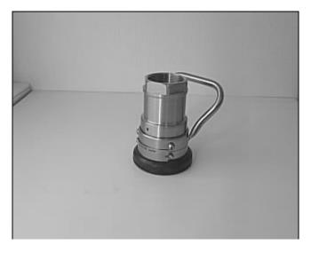
Finally, make a visual inspection that everything is in it's place. Do also a test connection / disconnection with a tank unit that not has any fluid inside. If the coupling works alright you are ready to mount the hose unit on your hose again.
