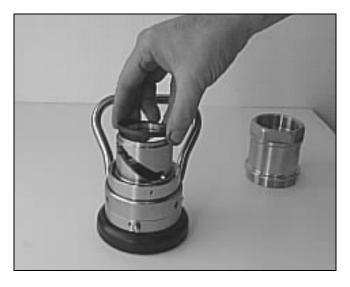
Remove the Teflon® bushing on the top of the coupling body.
