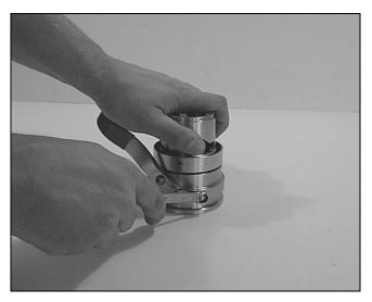
Change the three shafts (pos.18), locking nuts (pos.19) and rollers (pos.17) to new ones.
