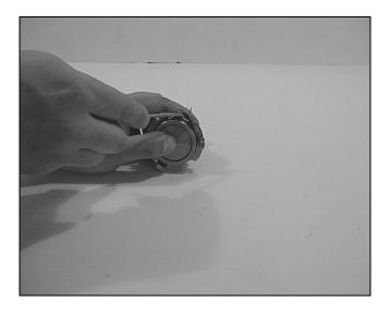
Change the O-ring (pos.6) on the driving plate front side. Use grease on O-ring.
