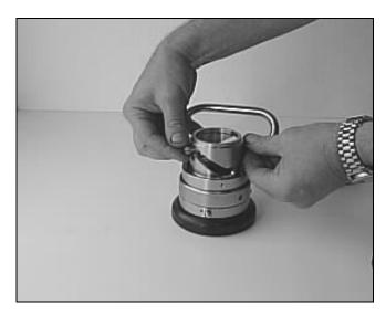
Remove the two shafts for piston guide and the two cylinder Teflon® bushing
