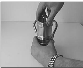
Mark the position of swivel sleeve against swivel ring with an Ø8 mm pin.
